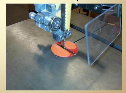
Only make adjustments while the motor is at a dead stop.
