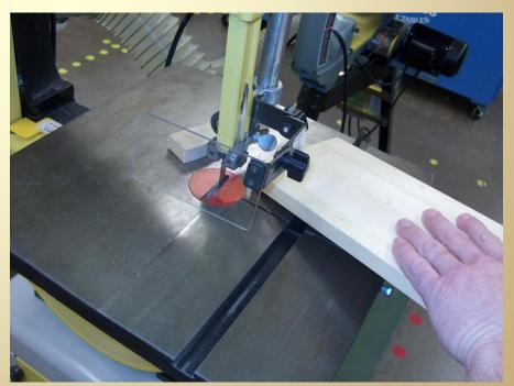
You may tilt the table to cut bevels on the band saw.
