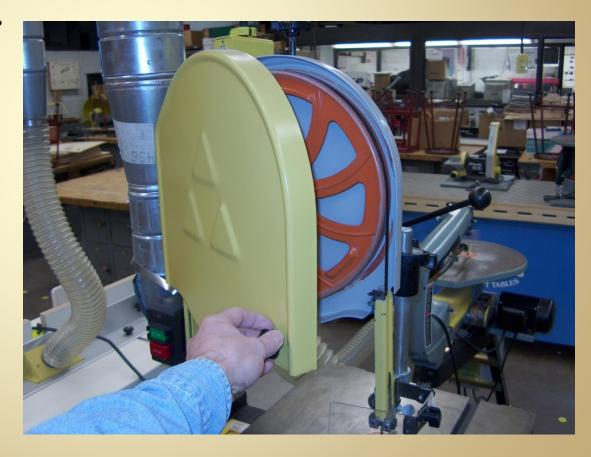
Check the blade for proper tension and check to make sure the teeth are pointing downward towards the table.
