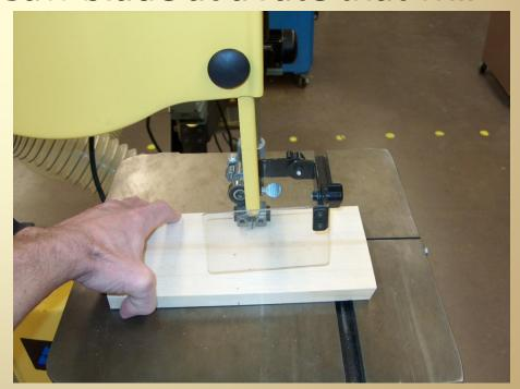
If you have to back out of a long cut shut the machine off and let it come to a complete stop before
