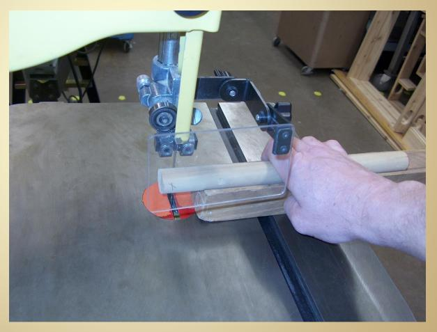
You may use the miter gage to help you cut miters or to just guide the material as you cut.
