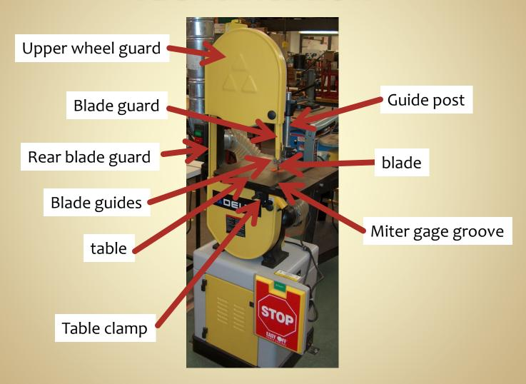
The band saw can be used for cutting curves, irregular shapes and straight cuts.
