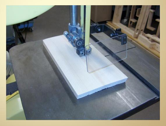
Allow the machine to come to a complete stop before leaving the saw.
